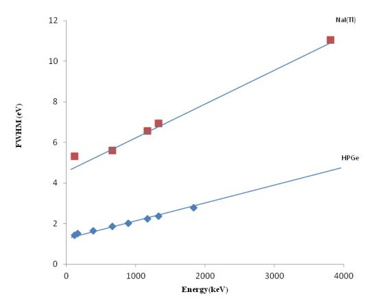
Figure 2. Resolution of HPGe detector and Nal (TI) detector as function of energy.
